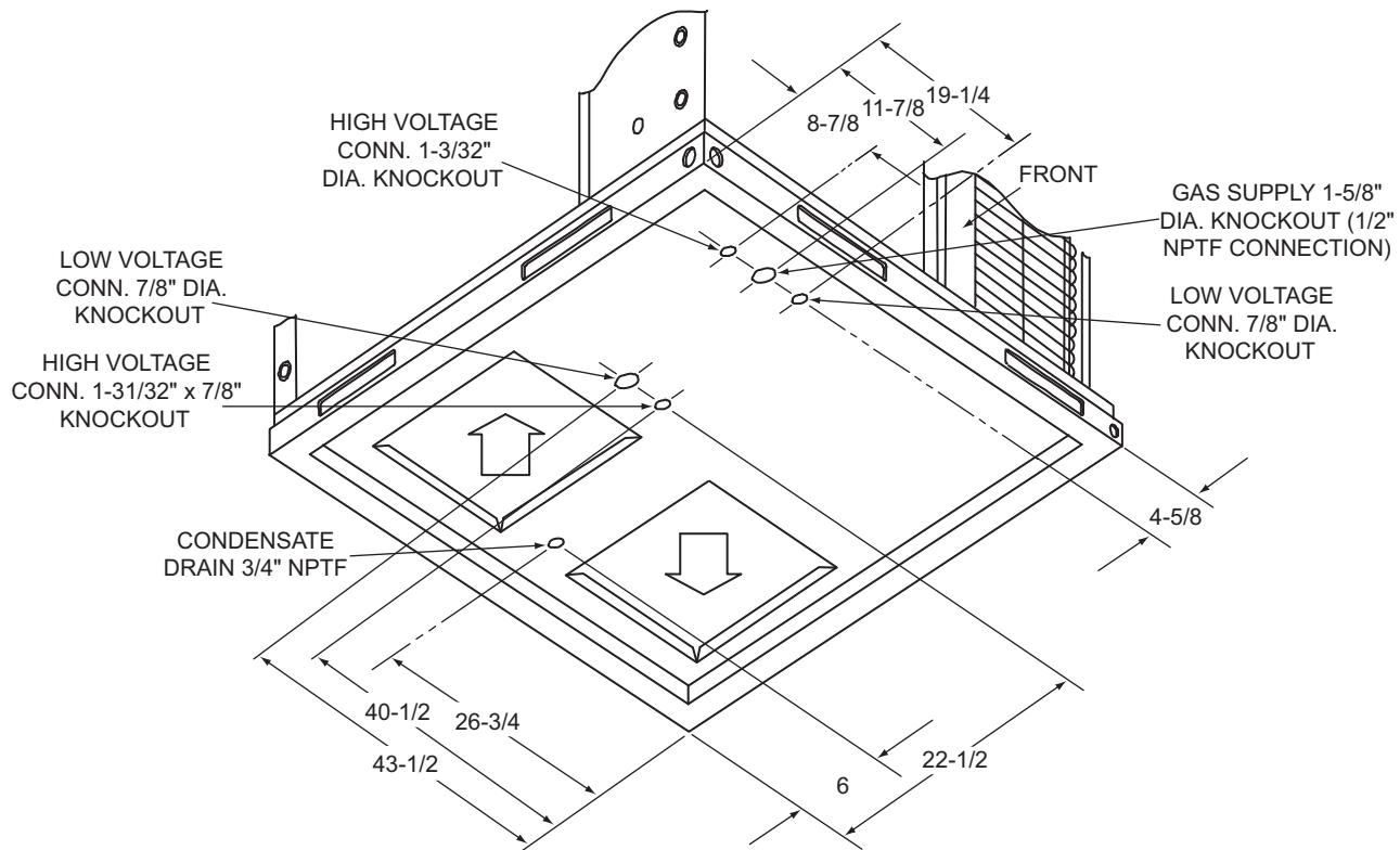
**Unit Dimensions Back and Bottom**
