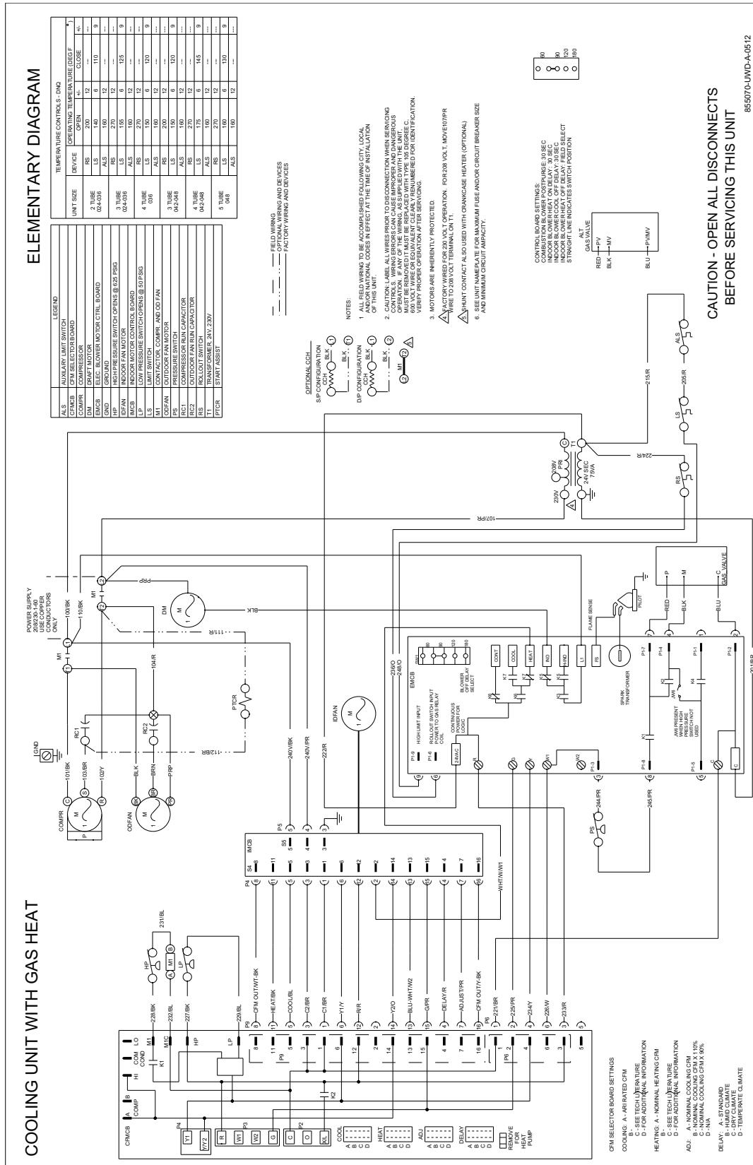
Typical DNQ024-048 Cooling Unit with Two Stage Gas Heat 208/230-1-60 volt Wiring Diagram
