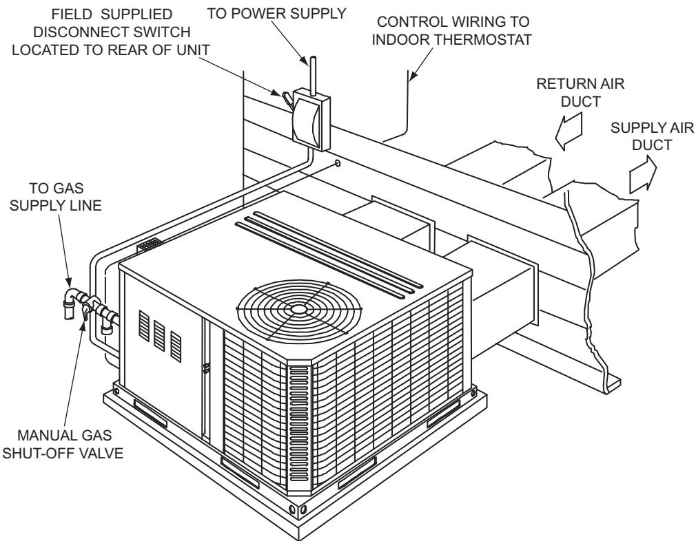
**Unit Typical Roof Curb Installation (Gas Model Shown)**
